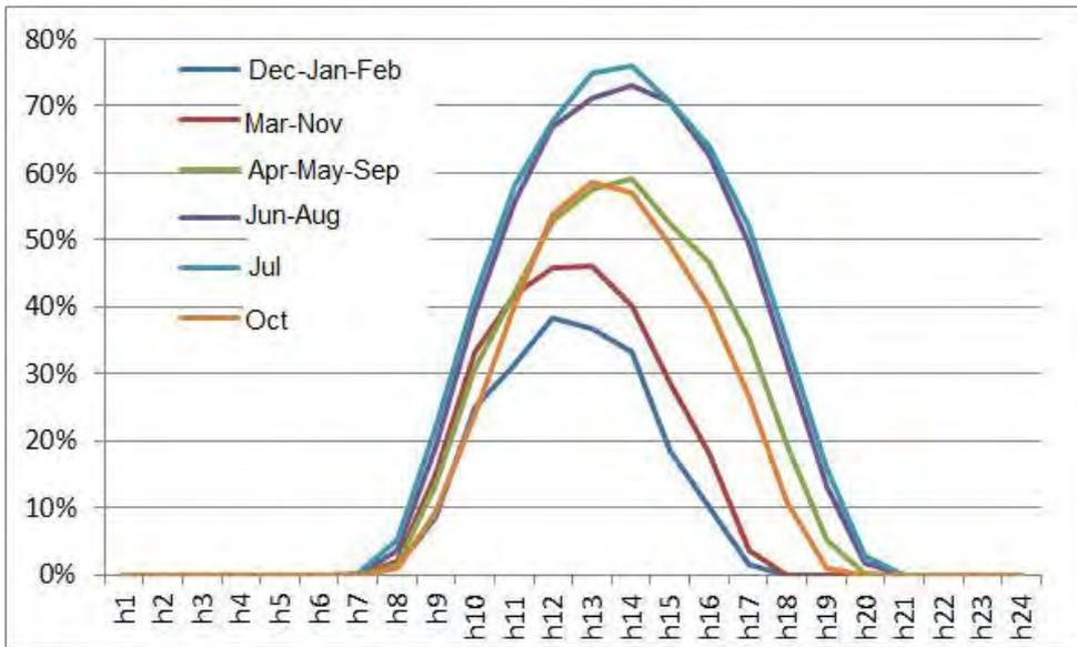
**Table A. 1: Capacity coefficient for small-scale hydro (HTSO, 2009)**
