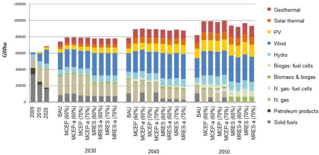
**Chart 12: Development of installed capacity per fuel for each scenario (Energy Roadmap to 2050)**
